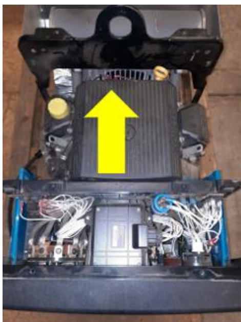
Figure 1 - Bobcat machine from above, arrow indicates solenoid location
