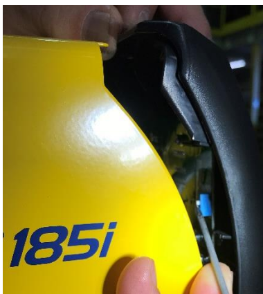
Figure 3 - Service mode switch
