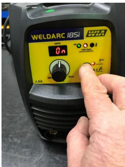
Figure 4 - Switch in to Service mode
