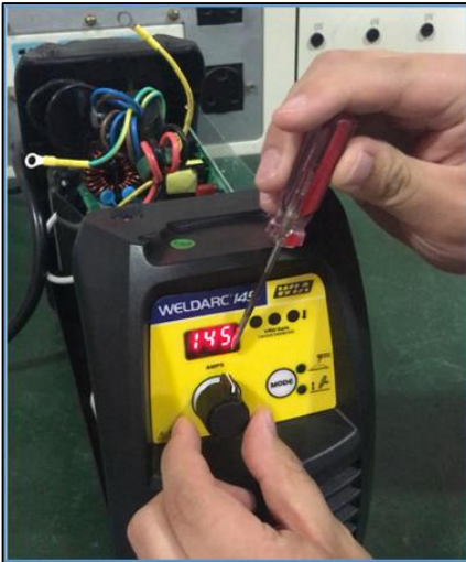
Figure 2 - Rotation of current selection knob
